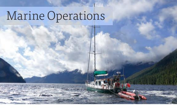
OUR DEDICATED RESEARCH VESSEL, *Achiever*, is a Transport Canadacertified 70 ft, steel hulled sloop that operates seven months a year on the BC coast. The boat can be fit to provide observer platforms, oceanographic equipment, freezer space, and other research requirements. It can accommodate up to 10 guests and has substantial water and fuel capacity. *Achiever* is also central to Raincoast's ability to administer and monitor our commercial hunting tenures in the Great Bear Rainforest.
